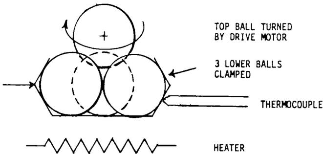
FIG. 1 Schematic of a Four-Ball Wear Test Machine
